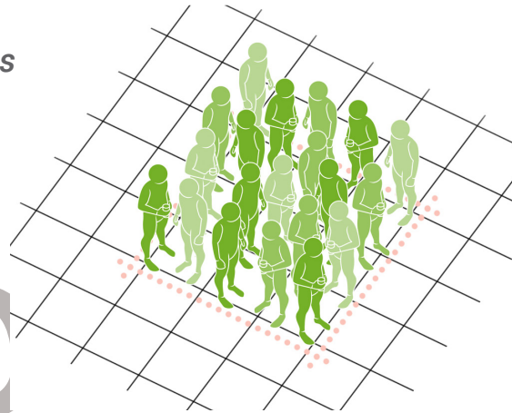
Standard operational mode (above): optimum concourse density of 20 persons per 10 square metres (0.5m 2 per person)
